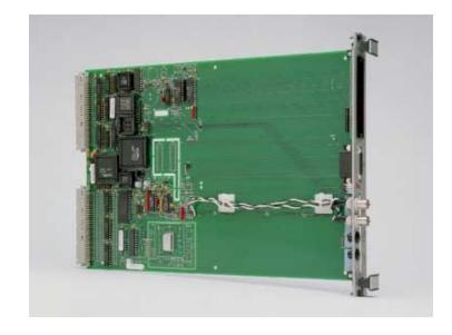
The VXI-SyncClock32 from Brandywine Communications provides precision time with zero latency to the host computer over the VXI bus. An on-board microprocessor automatically synchronizes the clock to reference signal inputs. The reference signal inputs can be 1 PPS, IRIG A or B and NASA 36 time codes. GPS and Have Quick inputs are optionally available. The clock can free run and be set by commands from the host over the VXI bus.
